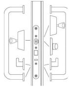
Automatically deadlocking lock for narrow profile doors. The sliding snib is released only when turning the key (or thumbturn).
