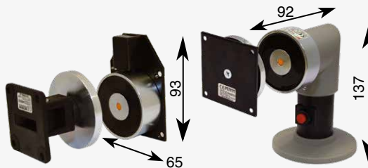
Wall magnets ABLOY® 7438, 7439 • Operating voltage 24VDC • Normal current 16mA • Hold open force 500 N
