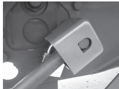
Landing Gear Lock Covers and locks the landing gear handle.
