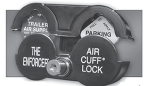
Air Cuff® Lock Prevents truck and trailer brakes from being released.
