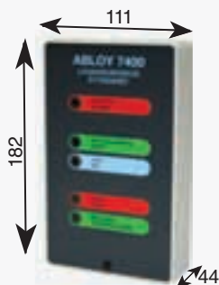
Control unit ABLOY® 7400 • Supply voltage 230 VAC • Output voltage 24VDC • Max. output current 300 mA
