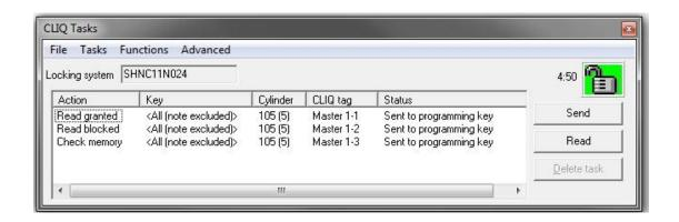
6. Now insert the Master Programming key in the lock (105 in this example). Wait until the re-programming is done. It may take some time. The key will indicate when the programming is done by making a long beep.
